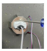
**INSTALL 21057 CONTROL PAD:** Determine the installation location of your control pad. Note the control module comes with a 7" long cord so the control pad will need to be located near the module. Drill a 2.125" hole and insert the control pad. Note, this version will only work with a 1/8" thick mounting surface.
