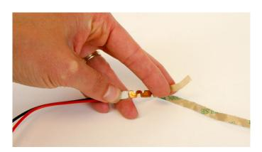
2. Press the light in place. Continue working along the light and peel the paper as you go. Only pull back a few inches at a time to prevent the tape light sticking to itself. The light can be bent at 90°, but should only be bent as shown below. Bending on the LEDs or smaller curves could result in damage to the light.
