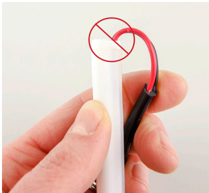
Do not bend right at solder joint
