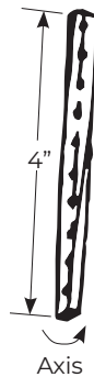
Do not twist more than 90° over the length of one 24V segment / Two 12V segments (4" total length)
