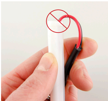
Do not bend right at solder joint
