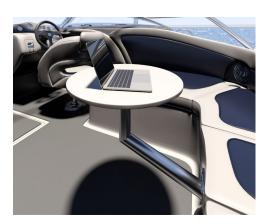
2. Slide the leg into the wall base. To remove the leg, pull the locking tab and slide the leg out.
