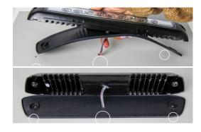
4. Press the light onto the rubber gasket then screw the light in place.
