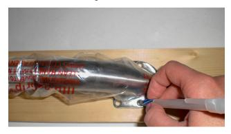
Wire the light based on the wiring diagram below, making sure the light is mounted at the top of the handle. Feed wires back into the hole and use silicone sealant around the wires to prevent any ingress of water. For added protection use silicone around the end caps.
