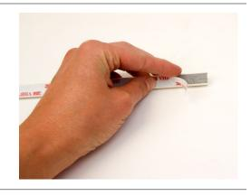
2. To install the light into the channel, start at the wire lead end and work the light into the channel going 6" at a time. The light should go into the channel pretty easily by just thumbing it in. Do not use any roller as that may cause damage to the LED circuit.
