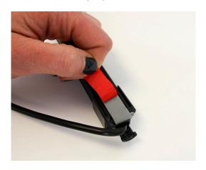
3. Wire the light following the wiring diagram below. The wire sleeve and grommet should be used for installations into metal backings to prevent damage to the wire. Additionally, silicone should be used around the wiring hole to prevent any ingress of water into the vehicle.
