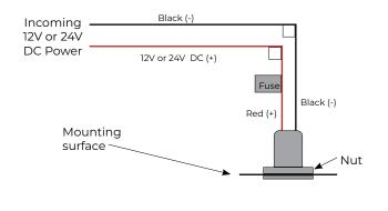
**3.** Feed the wires back through the hole<sup>1</sup> and tighten the nut<sup>2</sup> on the back of the light. If possible tighten the set screw<sup>3</sup>. The set screw is not required for installation but provides added support.
