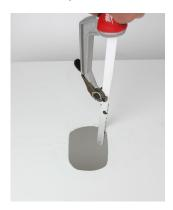
2. Insert the light into the hole and screw in using stainless steel
